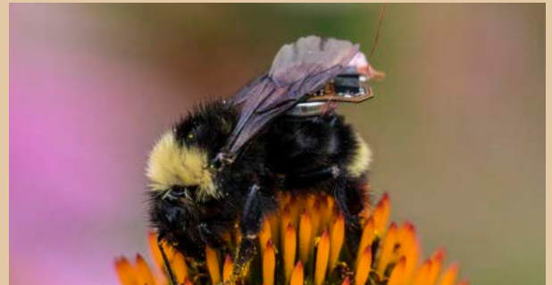
UW researchers have created a sensor package small enough to ride aboard a bumblebee. Photo by Mark Stone
