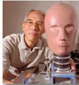
Randy Ching with a Hybrid III crash test dummy used in defining injury reference values.
