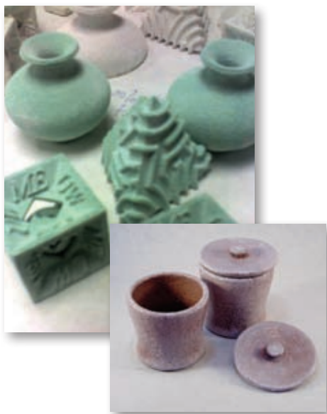
Sample parts printed using UWME ceramic powders, including fully glazed pots
