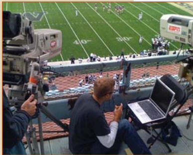
Jeff Siegmeth taking vibration measurements on Husky Stadium camera platform.
