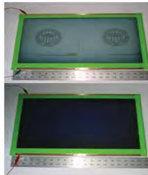
CIMS Electrochromic window of 12 x 20 inch size
