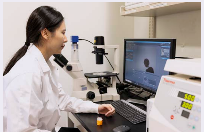
Top: Ph.D. student Runrun Chen applies a magnet to one side of a tube with magnetic microgel particles. Bottom: Chen uses optical imaging tools to study the shape of the microgel and check whether the iron oxide is successfully incorporated.
