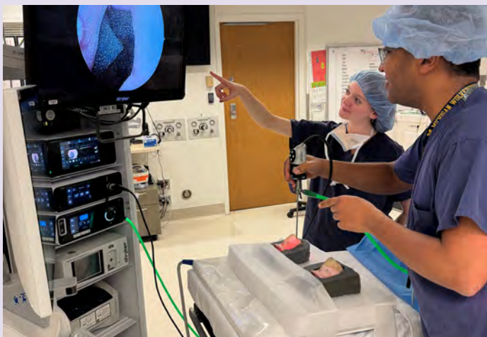
Nicole Gunderson and Dr. Waleed Abuzeid, UW Medical Center rhinologist and otolaryngologist, conducted an endoscopic survey of a 3D-printed sinus model to check the surgical completeness.
